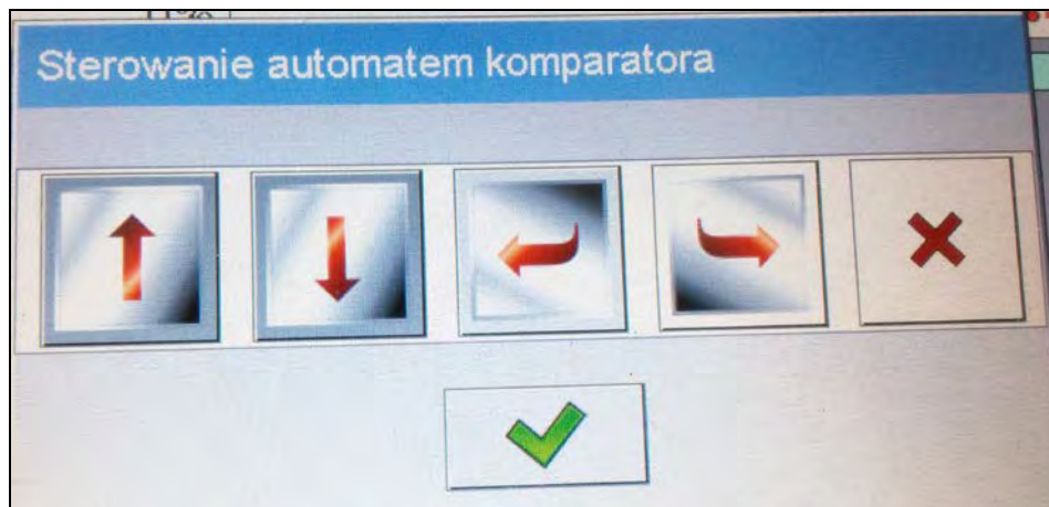
Keys and movements for slidable 2-position automatic comparator
